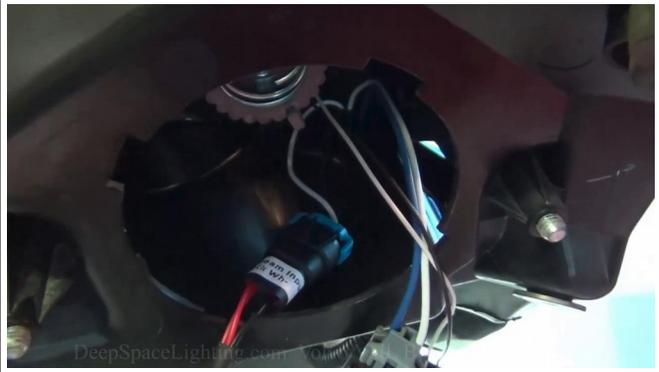
13. Connect single-pin wires from ballast to bulb adapter leads, and connect adapter harness *Ballast* connector to ballast input.
