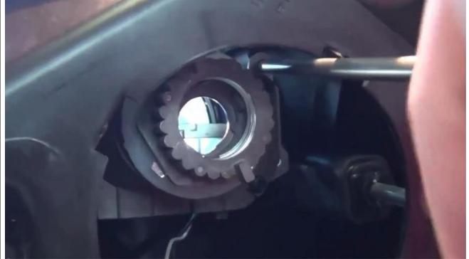
10. Connect *Low Beam Input* connector on adapter harness to connector removed from low beam bulb in step 9. Verify that plug is oriented correctly.
