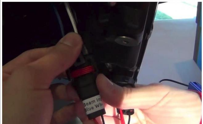
11. Connect adapter harness *High Beam Solenoid* connector to the connector attached to the bi-xenon projector (small red and black wires). Make sure connectors are inserted straight to avoid bending pins.
