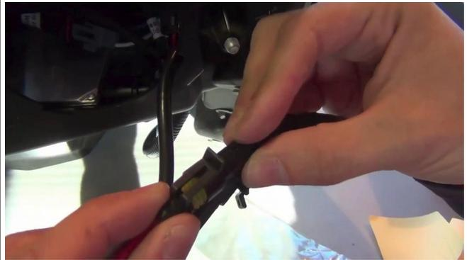
14. Connect bulb adapter to xenon bulb by aligning tabs on bulb, and twisting clockwise until locked. Do not use excessive force.
