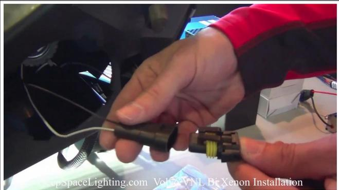
12. Unplug headlamp harness from high beam (lower) bulb, and connect the plug removed from the high beam bulb to the *High Beam Input* connector on the adapter harness.
