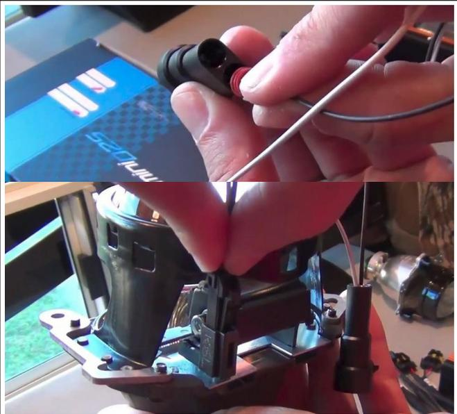
9. Loosely install bi-xenon projector in headlamp, starting but not tightening screws removed in step 3. Tighten screws once all 4 screws are started.
