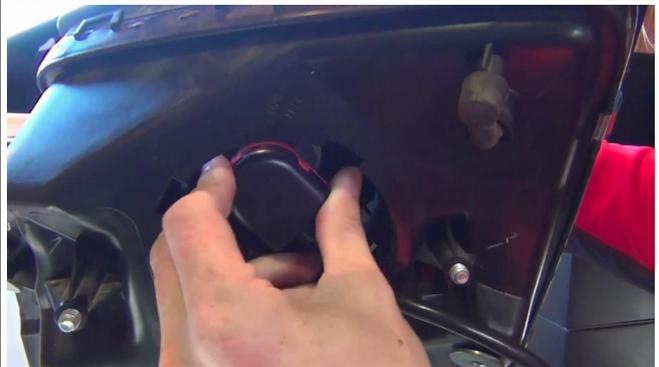
15. Secure ballast inside headlamp housing and reinstall headlamp housing onto hood. Reconnect headlamp harness to vehicle harness, and confirm headlamp operation with engine running.
