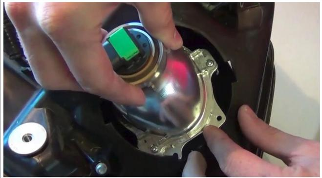
7. Remove bulb retaining nut and spring from bi-xenon projector. Remove xenon bulb from packaging. Install bulb into bi-xenon projector. There is a locating tab on both the bulb to orient the bulb properly. Re-install spring and bulb retaining nut.
